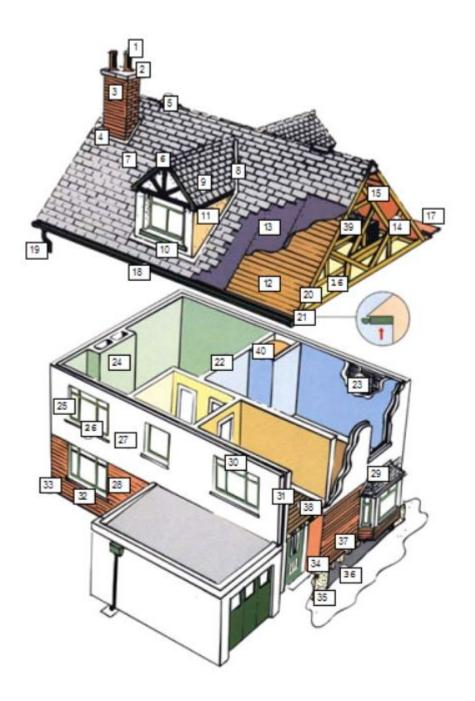
Ridge ventilation 5 Ridge board Slates/tiles 8 Valley guttering 9 Dormer projection Dormer flashing 10 Dormer cheeks 11 12 Sarking Roof felt 13 Trusses 14 15 Collar 16 Insulation 17 Parapet gutter Eaves guttering 18 Rainwater downpipe 19 20 Verge boards / skews 21 Soffit boards 22 Partition wall Lath / plaster 23 24 Chimney breast 25 Window pointing Window sills 26 Rendering 27 Brickwork / pointing 28 Bay window 29 30 Lintels 31 Cavity walls / wall ties
